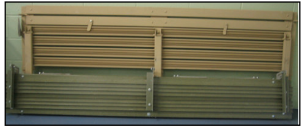
Fig. 3 – Current Troop Bench in Storage Configuration Requires 7.0 ft. 3 with AOM EMTB in Storage Configuration 4.66 ft. 3
