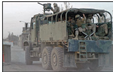
Fig. 12 – US Marines Sitting on Standard Issue COTS to Achieve Outward Seating Configuration
